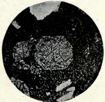
6.—Enstatite, transverse section. Ordinary Light. Showing form and cleavages.
